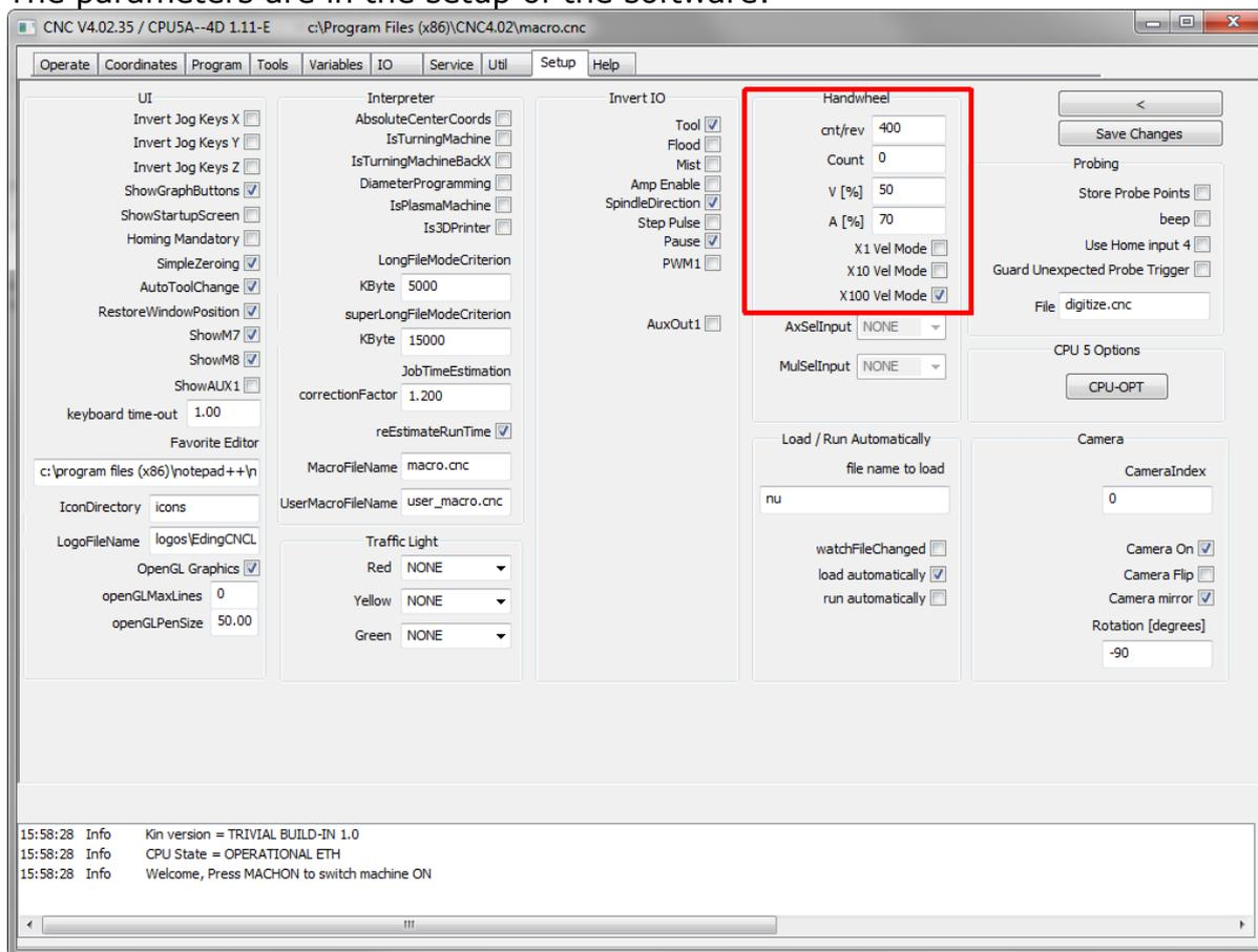
**Cnt/Rev:** The number of counts of the hand wheel for one revolution, usually 400 for most CNC hand wheels.
