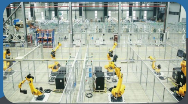
Factory area operation safety protection
