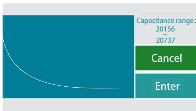
Because the capacitor is a sensitive to temperature and humidity of the environment, user should wait 3~5 minutes when power on to let the sensor and amplifier to reach a stable temperature.
