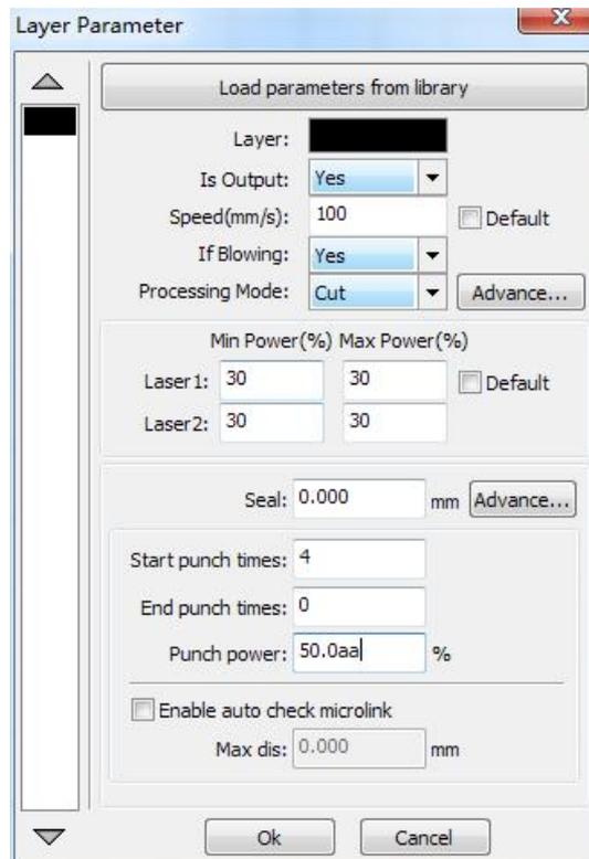
For laser piercing, the motion controller support CW piercing and pulse piercing mode. To set the piercing mode in the user parameters and layer parameters.
