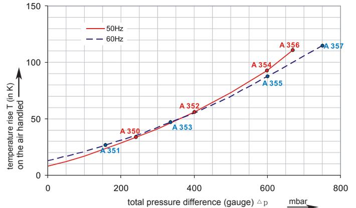
The performance curves are based on air at a temperature of 15 °C and an atmospheric pressure of 1013 mbar with a tolerance of +/- 10 %. The total pressure differences are valid for suction and ambient temperatures up to 25 °C. For other conditions please confer with us.
